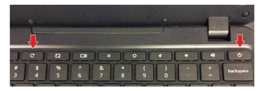
Press and hold the **Power button**. Then press the **Reload button** at the same time. Release both buttons.
